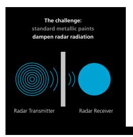
The coating must be optimized for autonomous driving:
